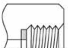
Sealing by gasket. Reference DIN 3852 Type Y
