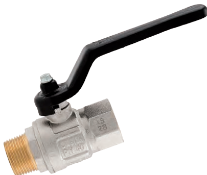
BSPT male/BSPT female (Rp ISO 7/1) - PTFE seal
